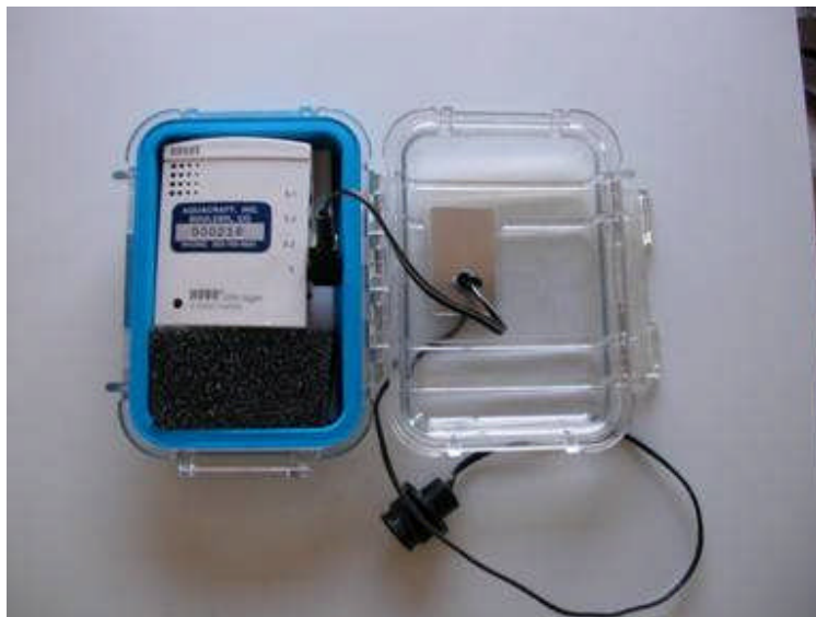
Figure 14. Close-Up of Water Logger in Case
