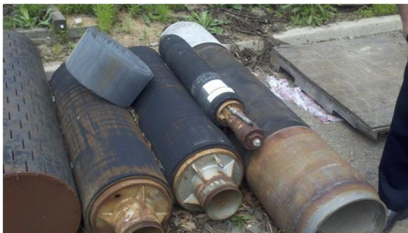
Figure 49. Use of packers to limit zones of poor water quality in a well. The packers are installed to limit portions of the aquifer. Packers cause problems for pump testers by blocking the access to the pumping water level.
