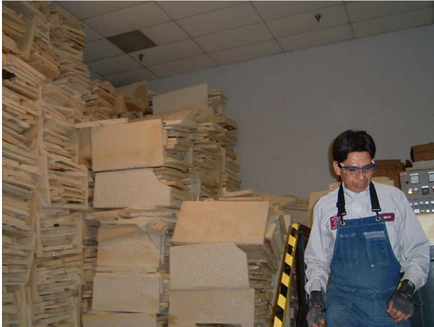
Figure B-4 Foam is Stacked, Then Loaded Into Equipment to Remove CFCs
