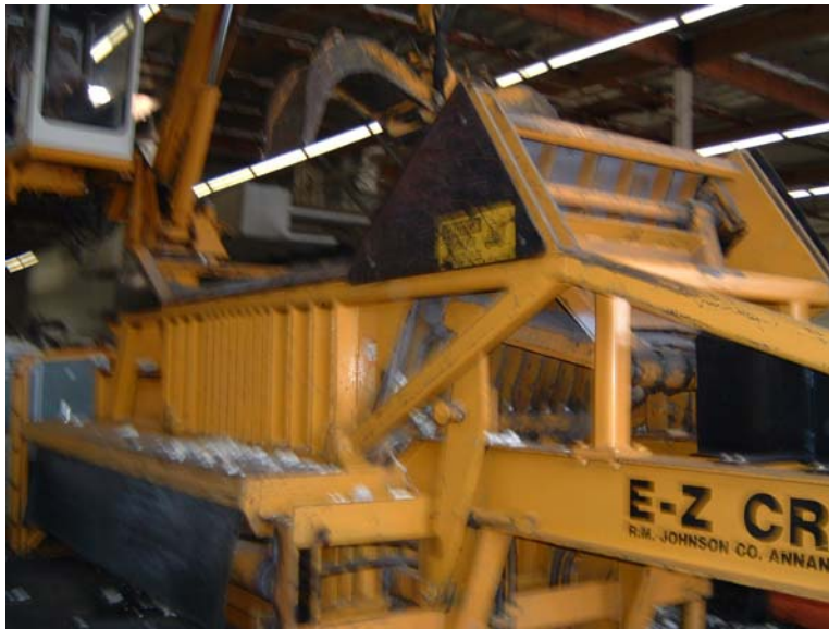
Figure B-12 Metal-crushing Equipment
