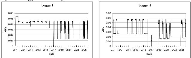
Figure 2.4 Logger I and J Plug Load Motion Sensor Field Measurements
