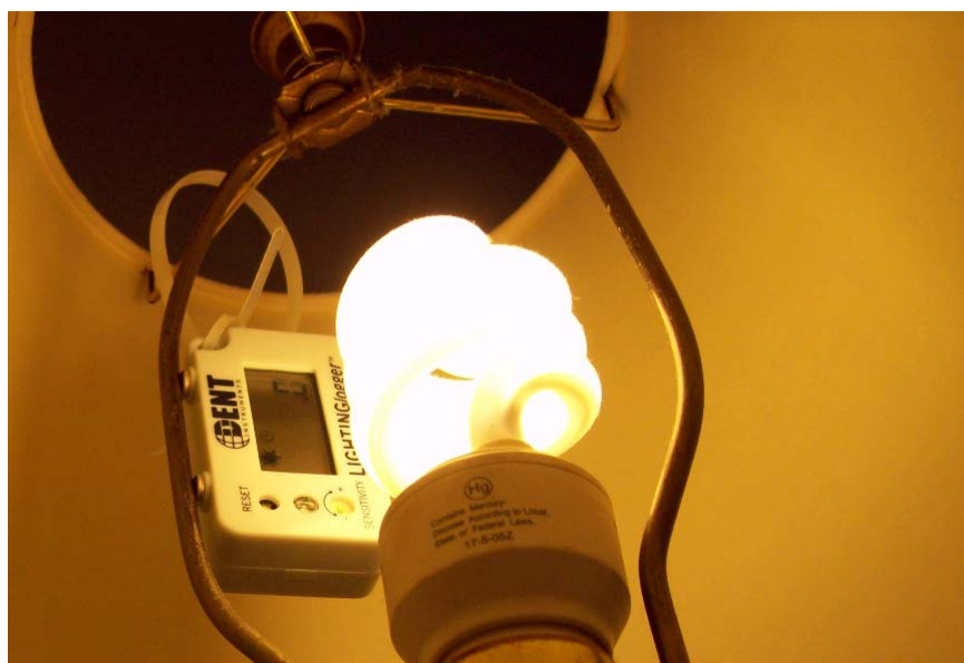
Figure E-7: LL Logger Installation in a Table Lamp w/ Zip Ties
