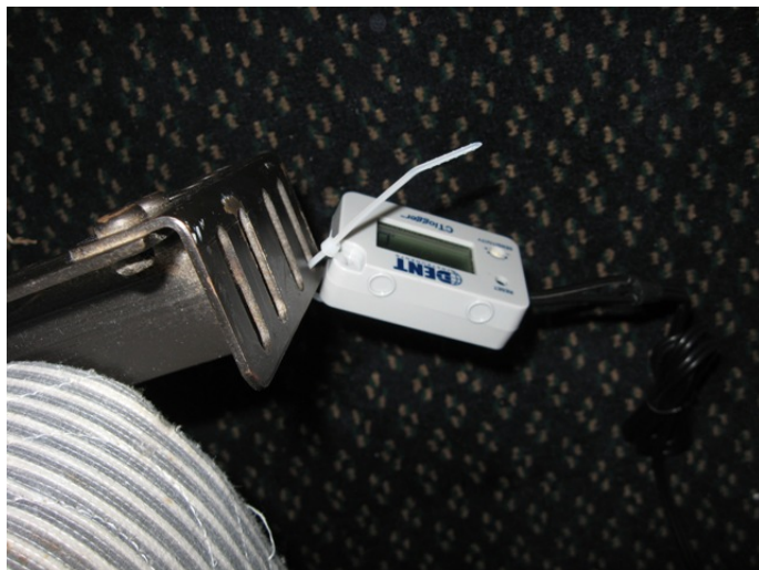
Figure E-8: CT Logger Zip tied to a Bed Frame
