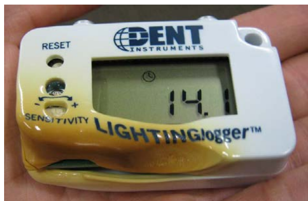
Figure E-12: Melted Lighting Logger
