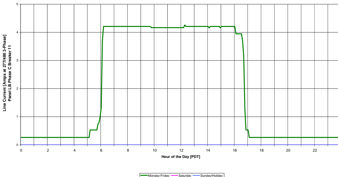
North Services Agency October/November 2003 Main Warehouse Shop Lights (ON) Average Daily Load Profile
