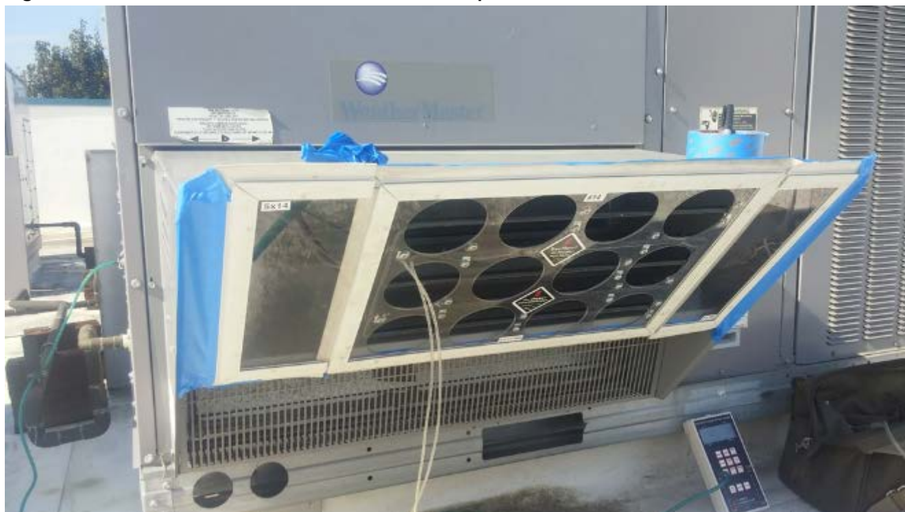
Figure 15. Trueflow outside air measurement set-up
