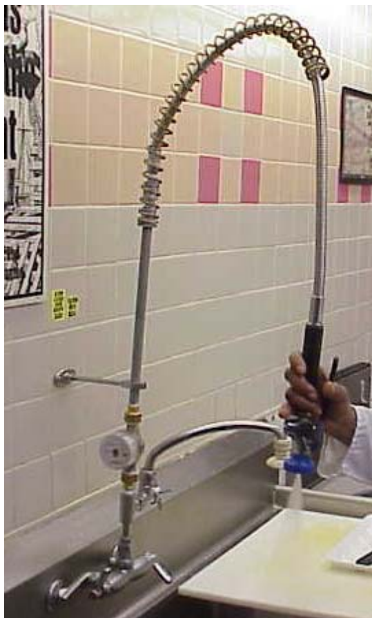
Figure 2-2: Metering setup for determining hours of use
