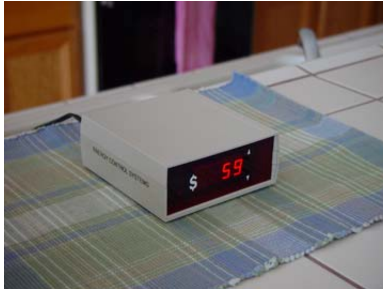
Figure 5. Energy Control Systems' Power Cost Display System with meter collar sensing
