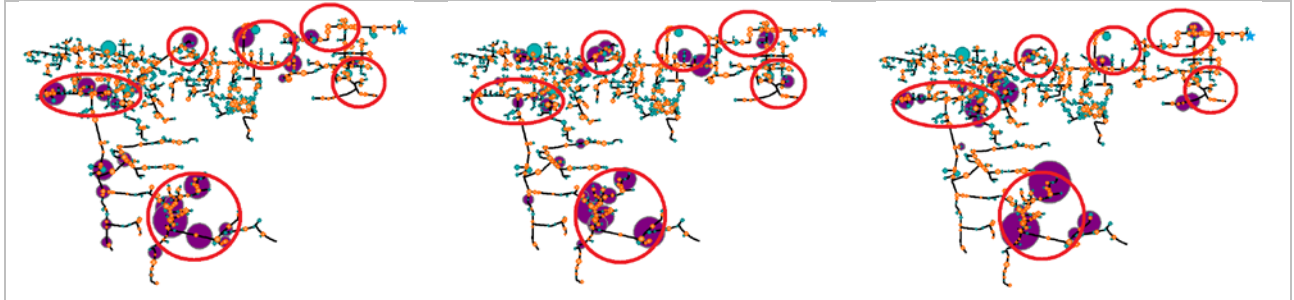
Figure 14. Simulation convergence for three simulation runs with the same settings. Regions that are chosen in all three runs for BESS installations are marked with red circles. The substation location for the feeder is indicated with a blue star on the top right. Results are for 75% PV penetration for feeder E for a day with clear morning and afternoon and partial cloud cover in the evening
