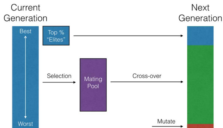
Figure 11. Each new generation is created through Genetic Algorithm (GA) operators: selection, cross-over and mutation. The next generation includes best individual(s) from the current generation (through elitism) and newly created individuals as a result of GA operators.
