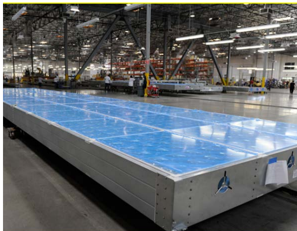
Figure 3 Later 7700 MegaModule, rated at 60 kW AC, manufactured in 2012.
