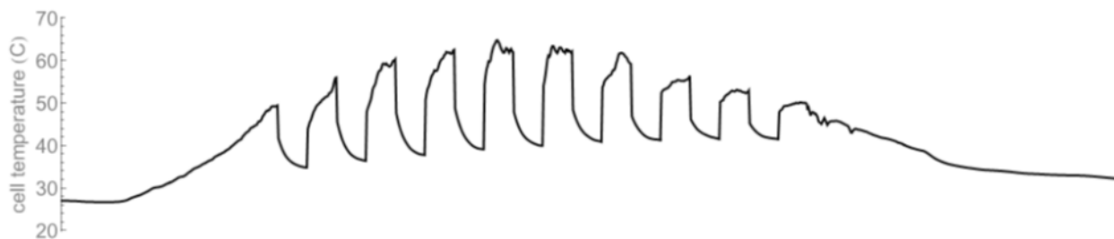
Figure 34: One set of validating experiments will involve periodically blocking sunlight with a shutter enables to exaggerate very damaging partly cloudy days. Causing cell failure in this way creates an experimental connection to the model that can support model-based absolute lifetime prediction.
