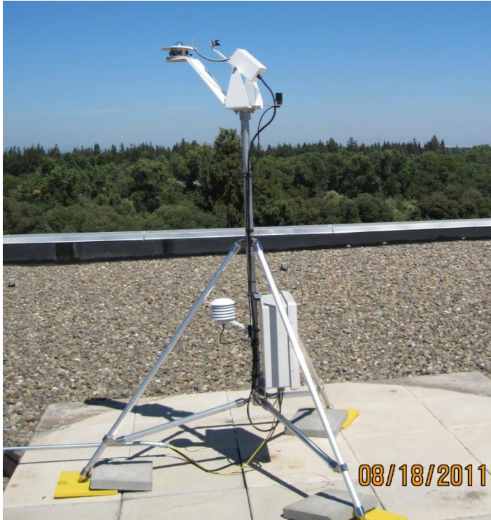
Figure 6-1. Primary station (rotating shadowband radiometer) located on roof of California State University Sacramento
