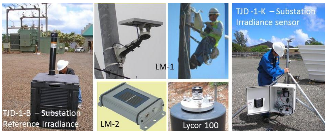
Figure 5-3. Examples of solar monitoring devices deployed in Hawaii and California
