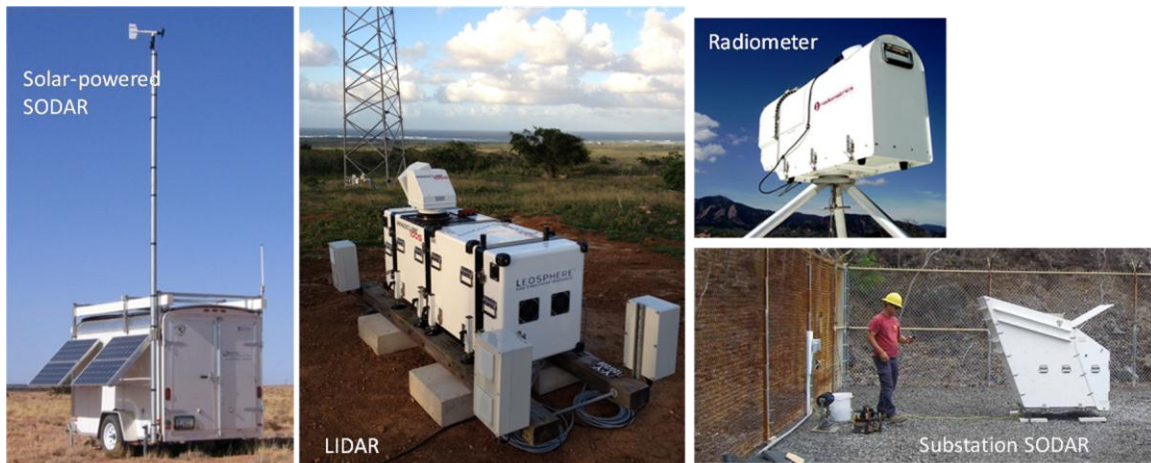
Figure 5-4. Remote wind monitoring sensors (SODAR and LIDAR) and temperature profilers (radiometer) deployed in Hawaii as part of the forecasting network (WindNET)
