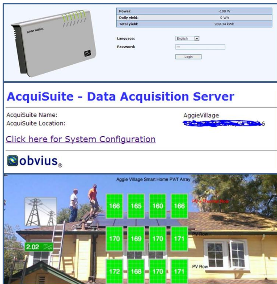
Figure 18: Screen shot of web based data server: top, SME Webbox; middle, Obvius smart panel; bottom, TiGo system
