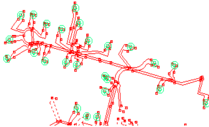
Figure 9. Detailed Feeder Model representation of a single distribution circuit and associated distributed roof-top PV systems shown in green.
