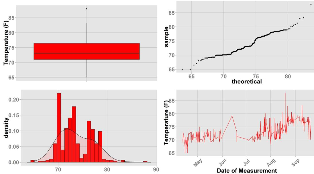
Figure 2.6: Detail of Return Air Wet Bulb Measurements Made by Technician: T00102
