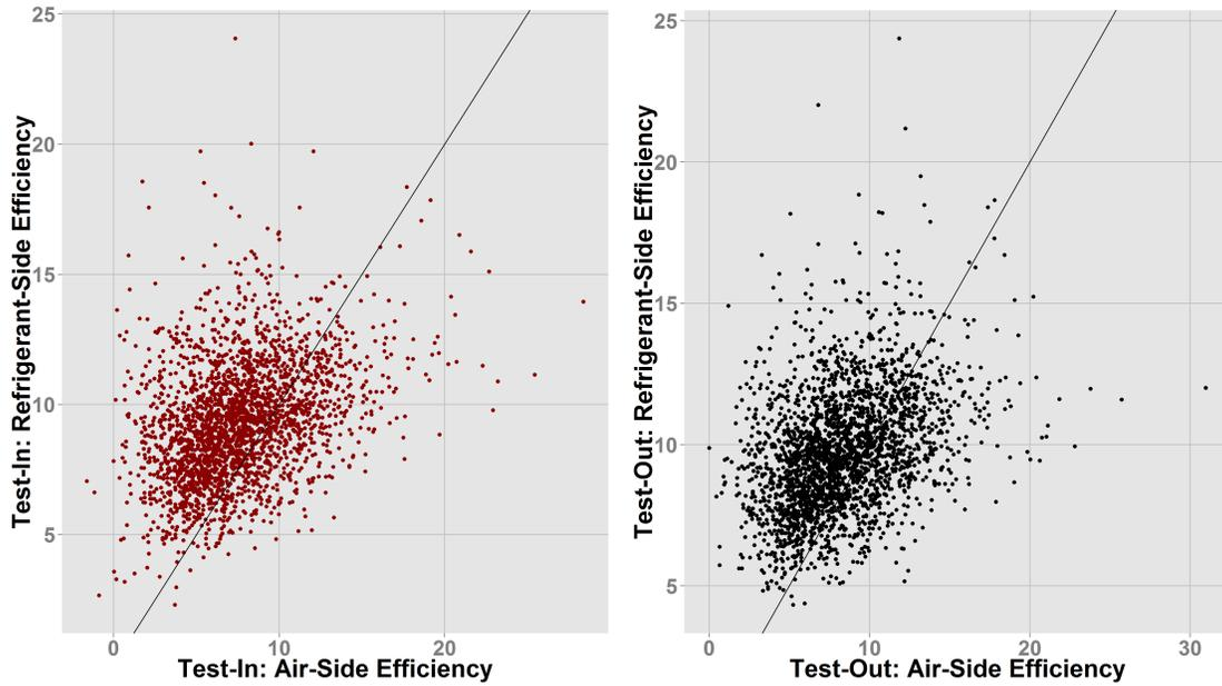
Figure 4.3: Comparison of Air-Side to Refrigerant Side In-Situ Efficiency Calculations
