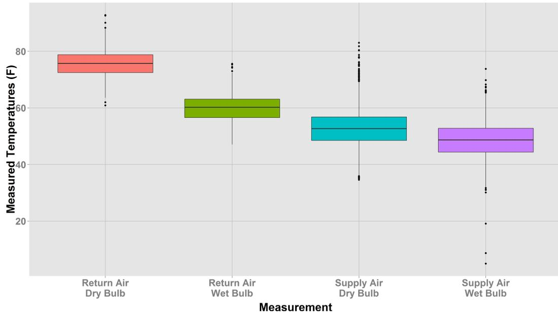
Figure 2.1: Box-Plot Summary of Air Temperature Measurement Data
