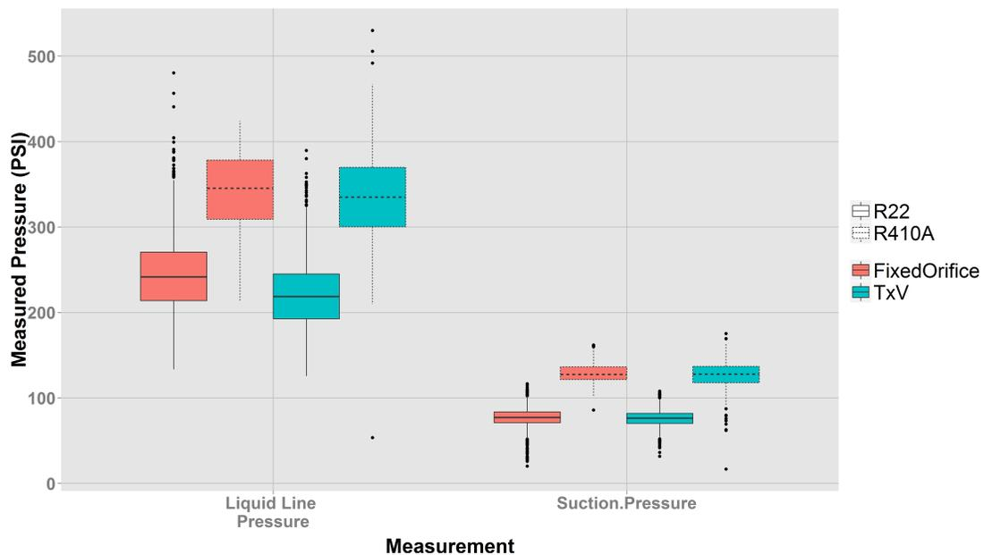
Figure 3.7: Box-Plot Summary of Refrigerant Pressure Measurements
