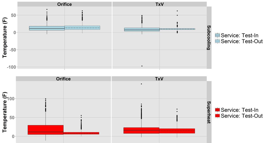
Figure 3.5: Comparison of Superheat and Subcooling Data by Metering Device and Test Conditions
