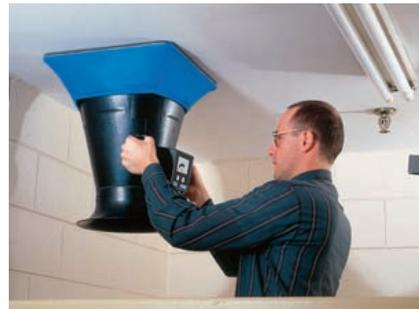
The LoFlo Balometer® Capture Hood is mainly used in residential or light commercial applications for taking measurements from 10 to 500 cfm (17 to 850 m<sup>3</sup>/h). The compact size allows them to be used where full size hoods would not fit such as over bathroom stalls or filing cabinets.
