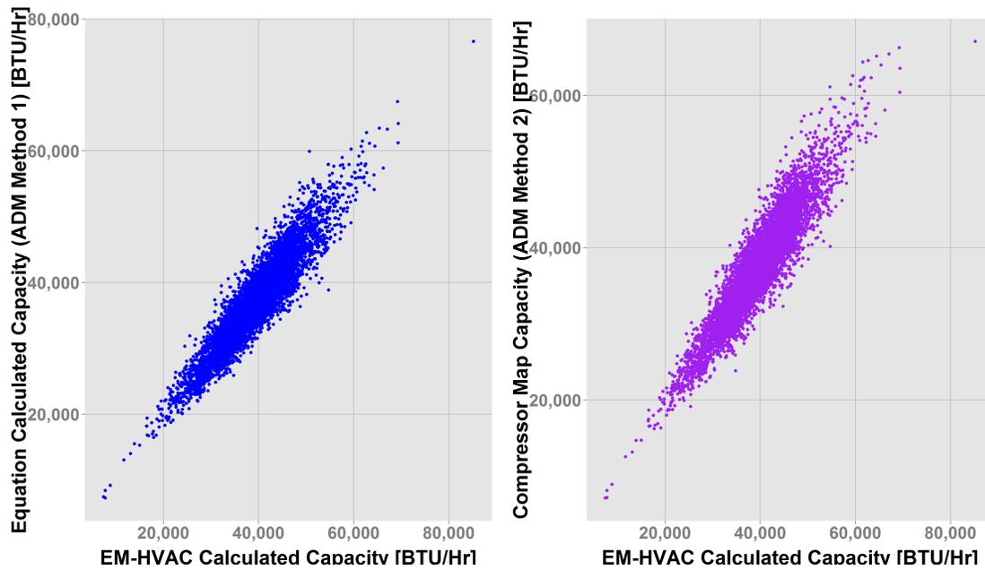
Figure 3.12: Comparison of System Load as Calculated By EM-HVAC to ADM's Calculations
