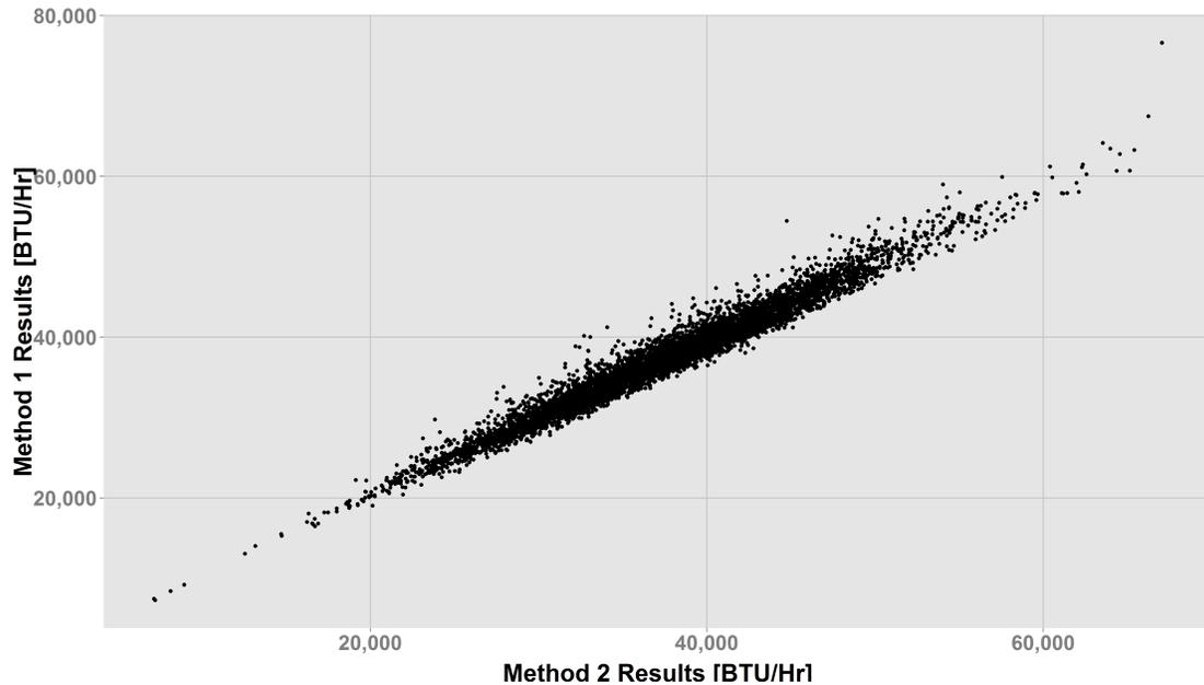
Figure 3.11: Comparison of Calculated System Load Between Equation 3.1 and Capacity Curves
