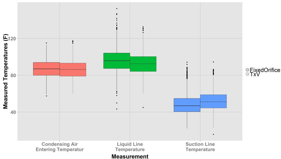
Figure 3.2: Box-Plot Summary of Refrigerant Temperature Measurement Data
