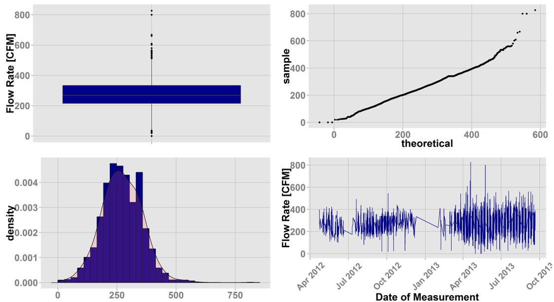
Figure 2.15: Distributions of "Measured" Air Flow Rate per Nominal Compressor Capacity (Default Observations Excluded)
