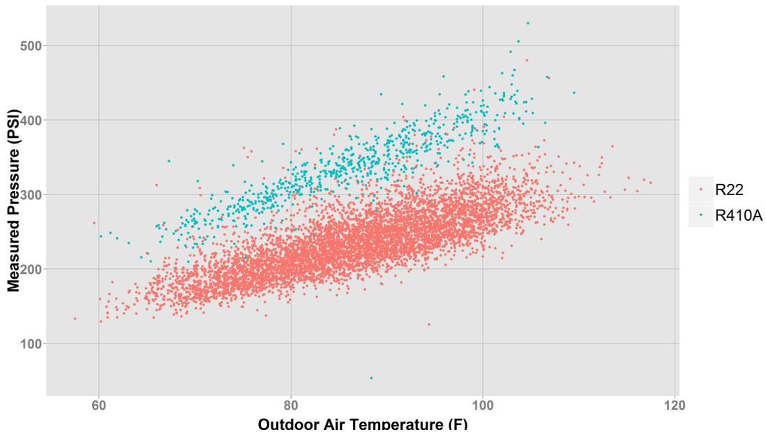
Figure 3.8: Correlation Between Refrigerant Liquid Line Pressure and Outdoor Air Temperature
