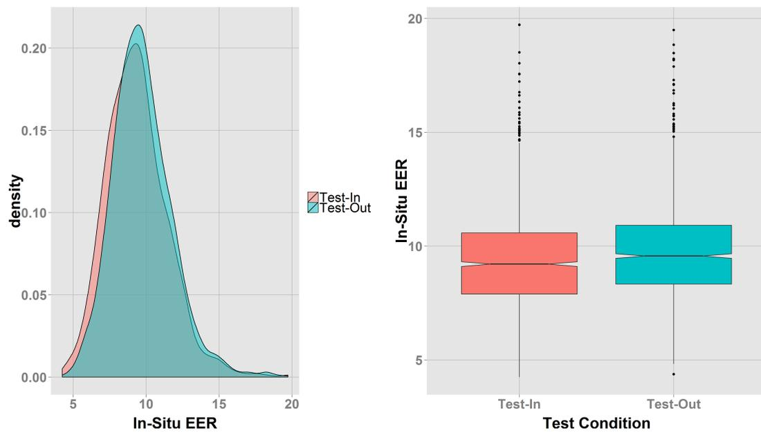
Figure 3.14: Comparison of In-Situ EER Measurements Between Test-In and Test-Out (Refrigerant Side)
