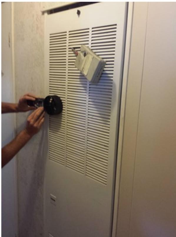
Figure 2.12: Typical Volumetric Air-Flow Measurement
