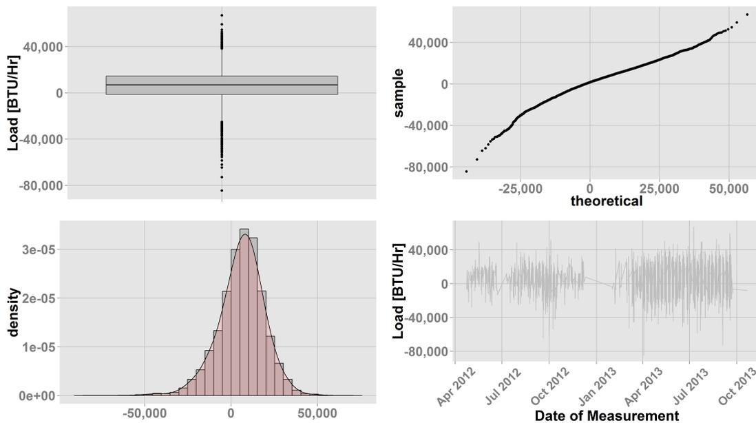
Figure 4.2: Difference Between Air-Side and Refrigerant-Side Load Calculations
