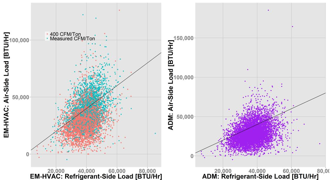
Figure 4.1: Comparison of Air-Side to Refrigerant Side System Load Calculations
