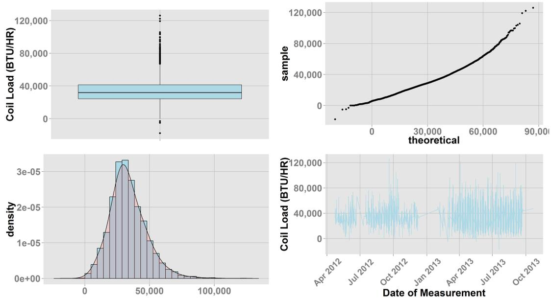
Figure 2.16: Detail of "Measured" Air-Side Capacity (Evaporator Coil Load)
