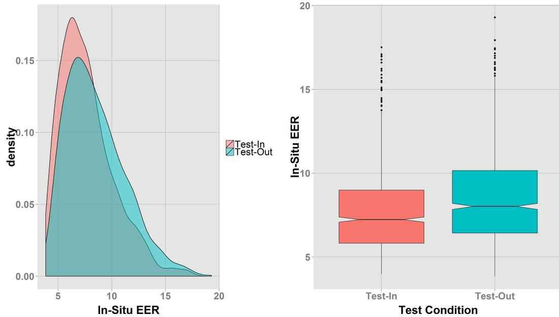
Figure 2.18: Comparison of In-Situ EER Measurements Between Test-In and Test-Out
