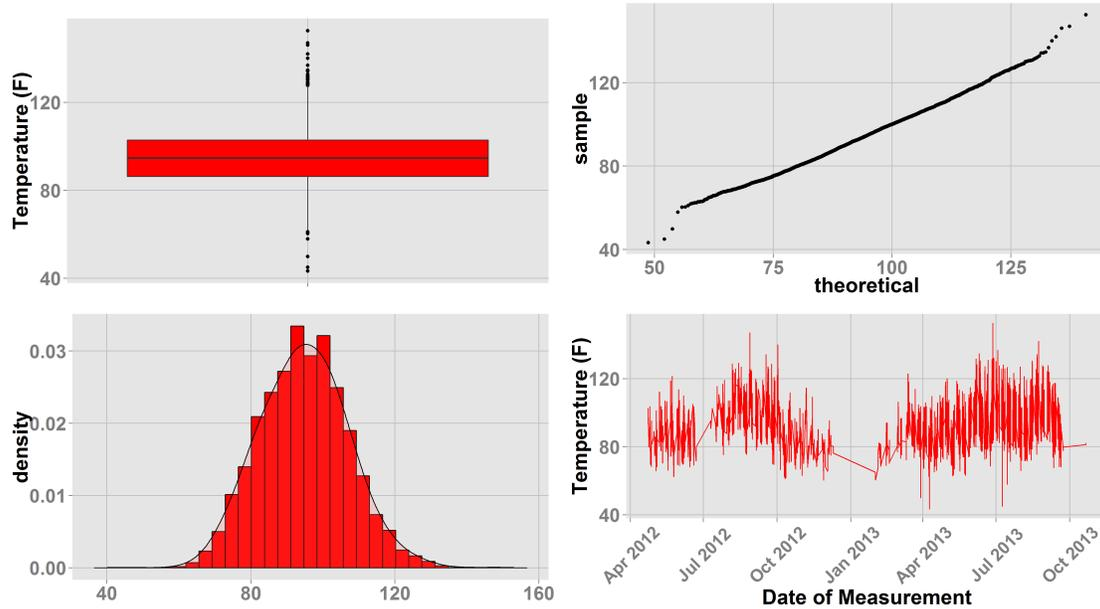
Figure 3.3: Detail of Measured Liquid Line Temperatures
