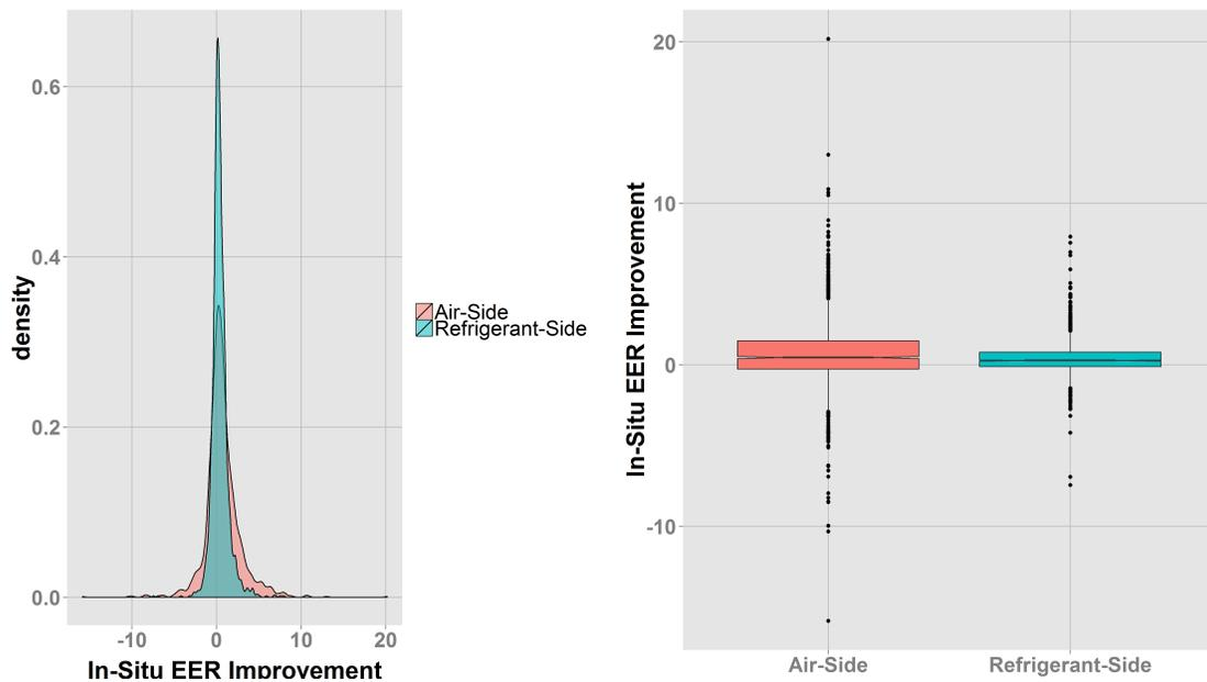
Figure 4.4: Comparison of In-Situ EER Improvement Between Refrigerant Side and Air-Side Metrics
