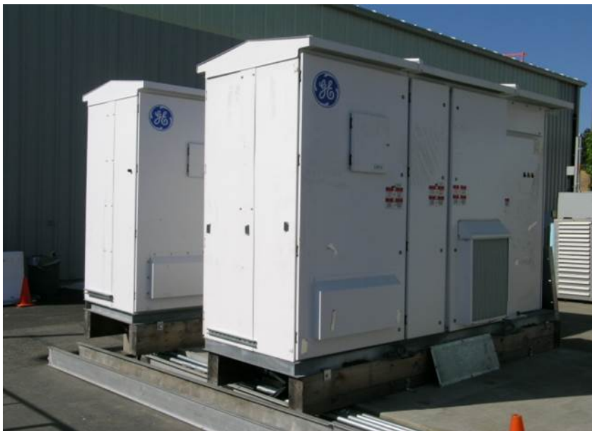
Figure 10 MW-scale electronic load at PG&E Applied Technology Services in San Ramon CA
