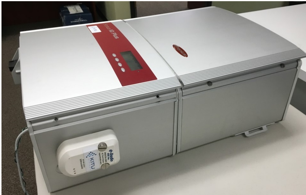
Figure 6-1, Example of Direct Communication Module Placement
