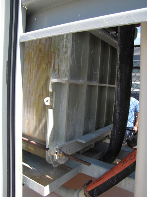
12 - Back side of Unit 3 top cells where leak occurred
