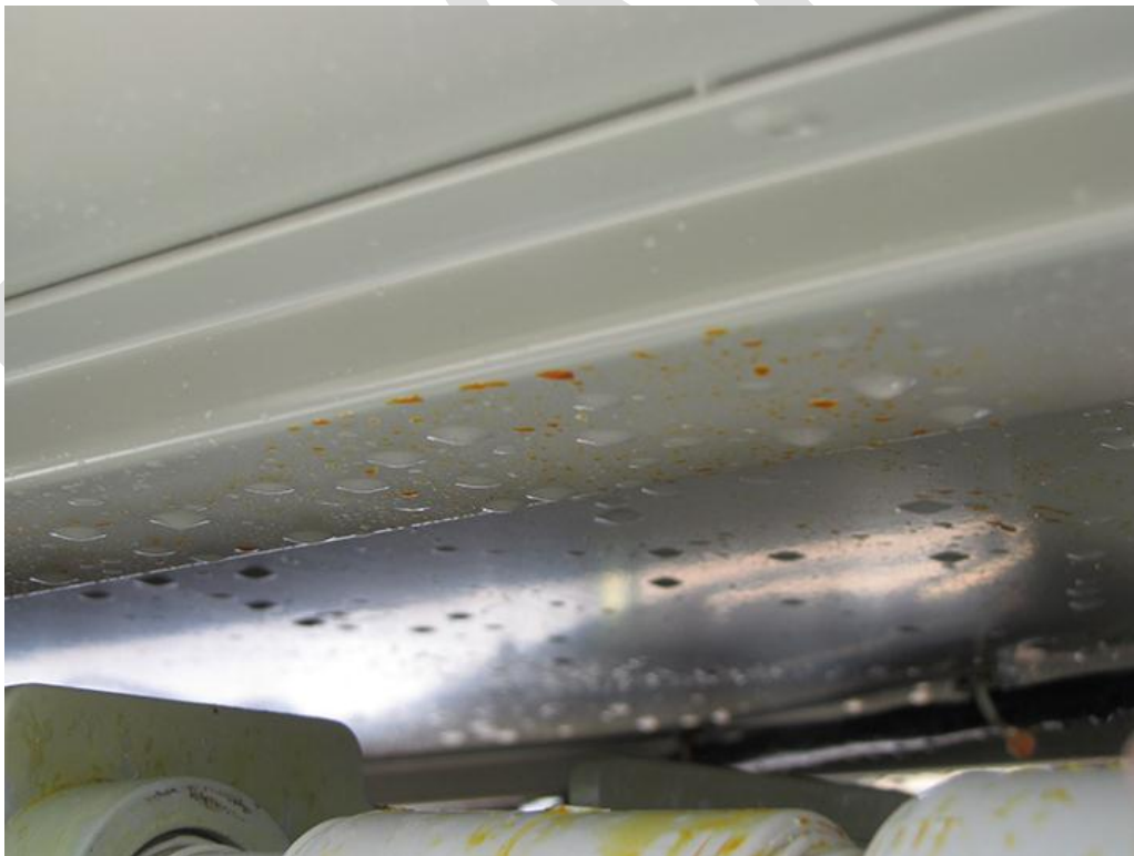
13 - Electrolyte residue along on top part of container
