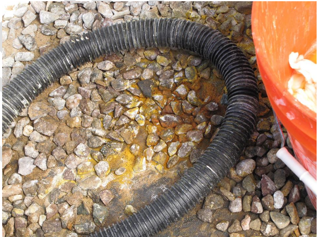
4 - Unit 3 Electrolyte external spill
