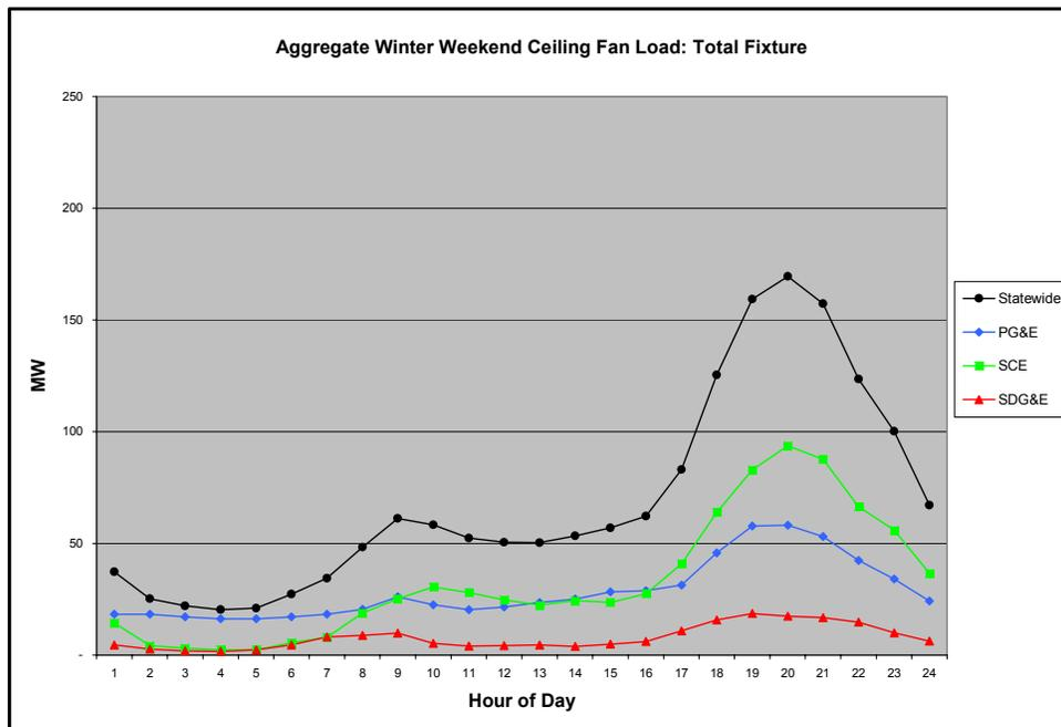
**Figure 37 Winter Weekend Ceiling Fan Total Fixture System Load**
