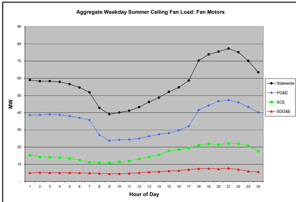
Figure 23 Summer Weekday Ceiling Fan Motor System Load
