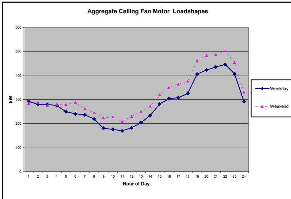
**Figure 47 Ceiling Fan Population System Load**
