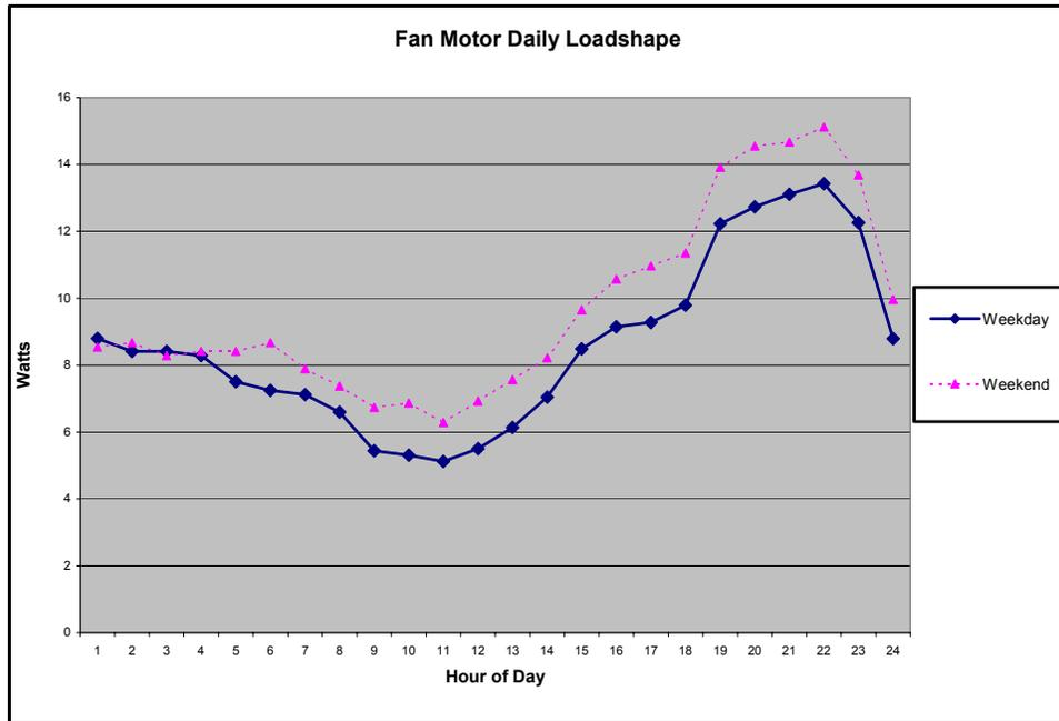
**Figure 45 Average Fan Motor Loadshape**
