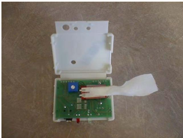
**Figure 13: HOBO Vibration Logger Modified with Ribbon**
