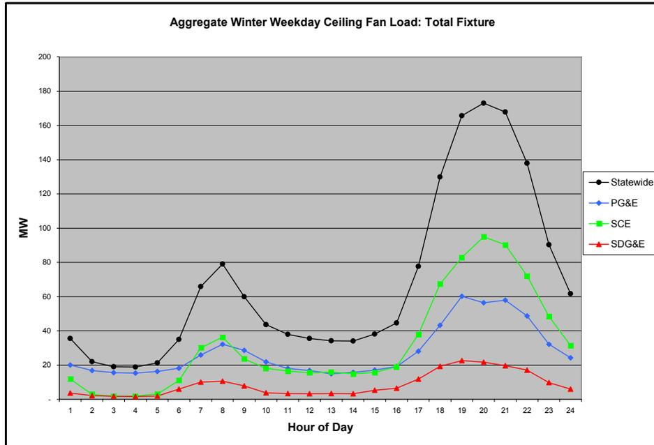
Figure 34 Winter Weekday Ceiling Fan Total Fixture System Load
