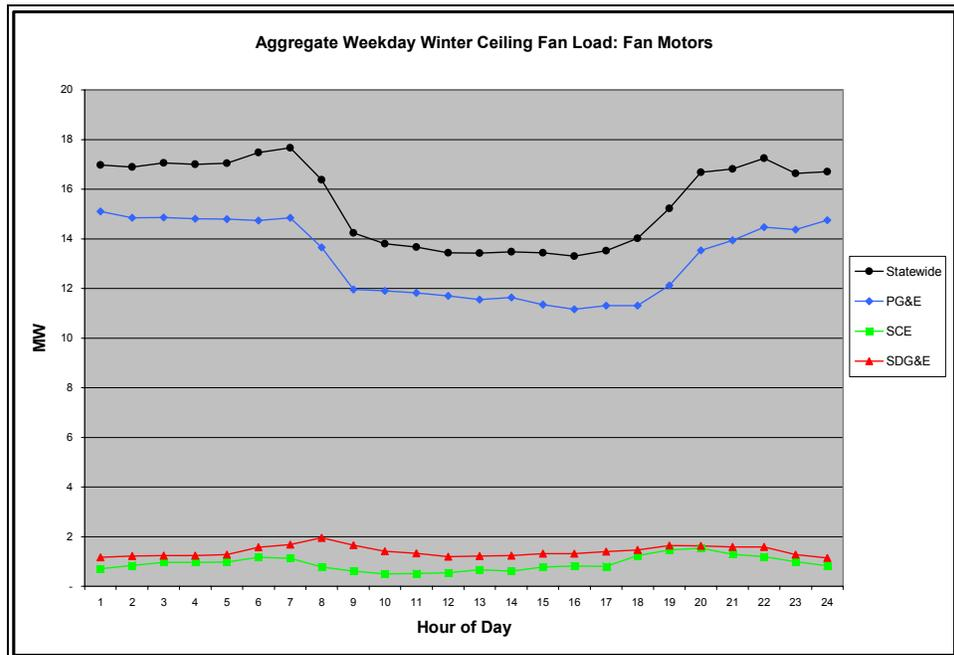
Figure 35 Winter Weekday Ceiling Fan Motor System Load
