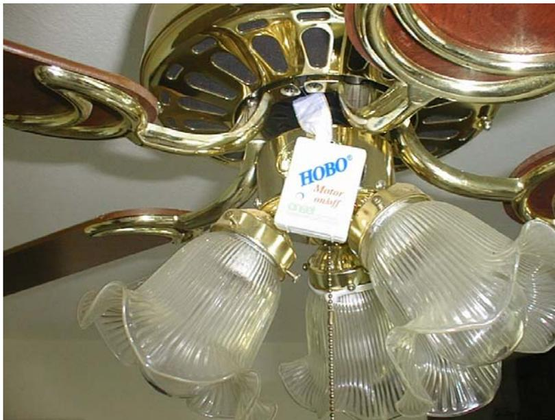
**Figure 14: Primary Motor Logger Mounting Location**
