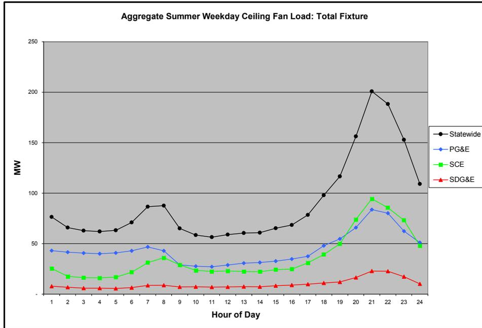
Figure 22 Summer Weekday Ceiling Fan Total Fixture System Load
