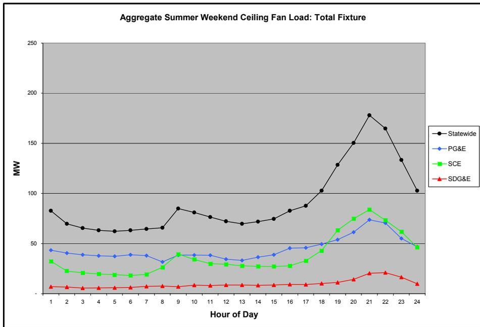
Figure 25 Summer Weekend Ceiling Fan Total Fixture System Load
