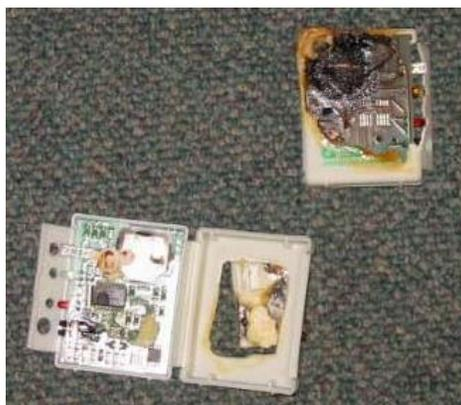
**Figure 16 Damaged Lighting Loggers**
