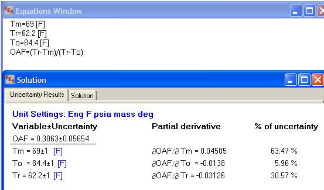
Figure 5. Outdoor Air Fraction and Uncertainty for 4-ton non-TXV Unit (004-1293)
