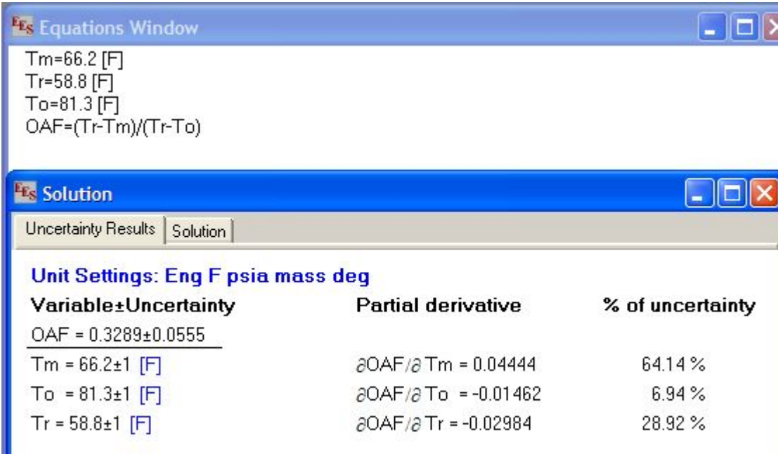
Figure 9. Outdoor Air Fraction and Uncertainty for 4-ton non-TXV Unit (004-1296)
