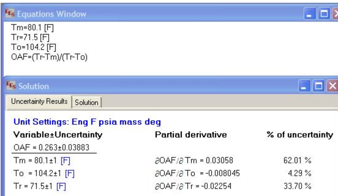
Figure 6. Outdoor Air Fraction and Uncertainty for 4-ton non-TXV Unit (004-1289)
