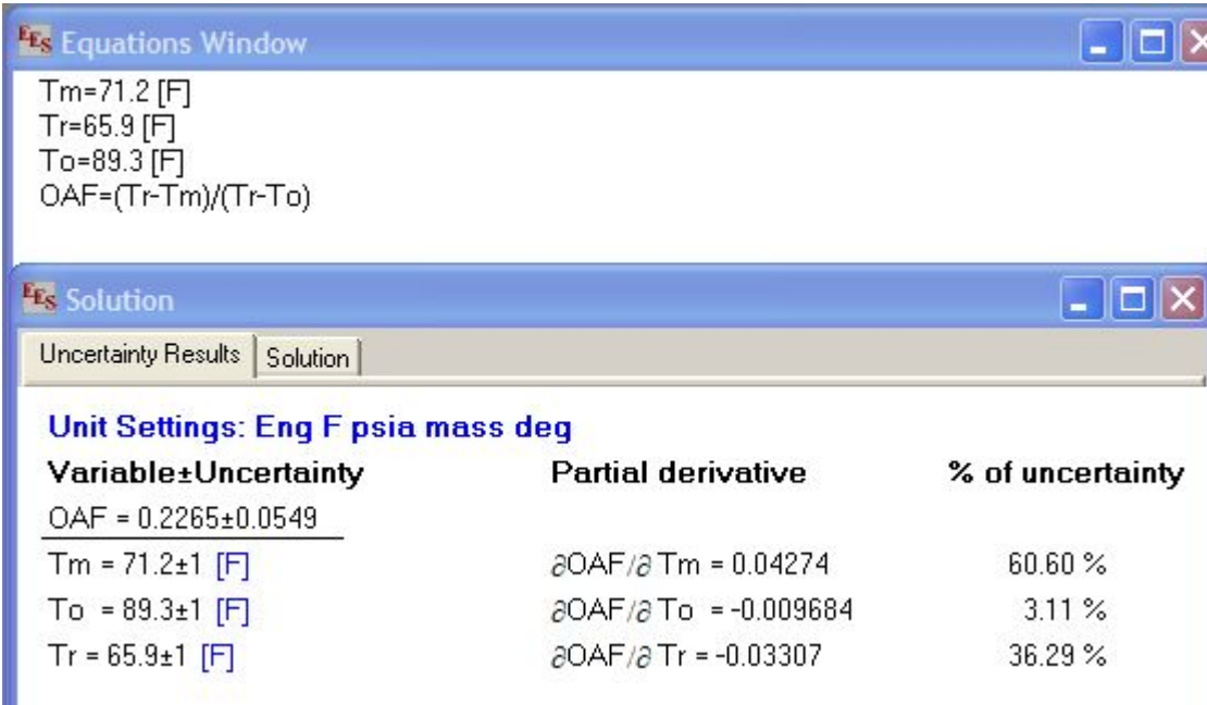
Figure 7. Outdoor Air Fraction and Uncertainty for 4-ton non-TXV Unit (004-1295)
